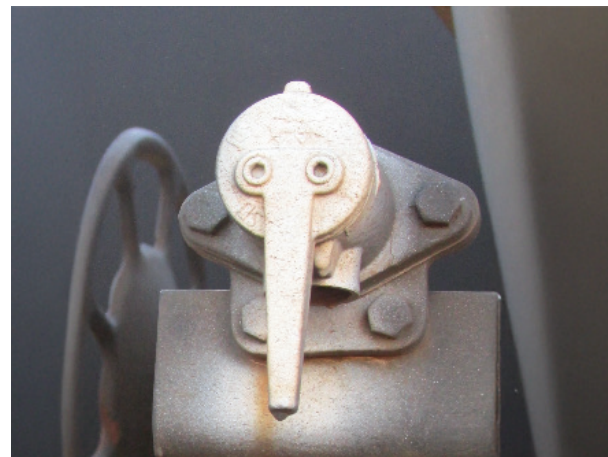
f. Vent valves, including the proper positioning of the vent valve during in-plant railroad operations
